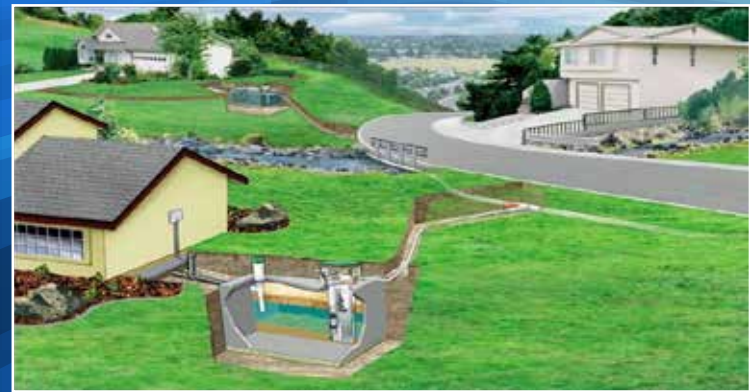
Septic Tank Effluent Pump (STEP) collection systems provide an economical alternative to conventional gravity collection systems in rocky, hilly terrain because they are shallow, small diameter pipe systems that don't require constant grade and they eliminate the need for manholes and costly lift stations. (Image by Orenco Systems)
