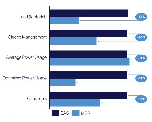
While MBR technology can have a reputation for higher energy consumption compared to conventional activated sludge systems, focusing on the broader picture reveals significant advantages including the elimination of secondary clarifiers, optimized aeration, enhanced bio-gas recovery, and superior water quality.
